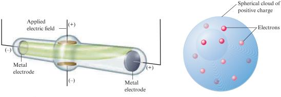
**Figure 2.8** Deflection of cathode rays by an applied electric field.
