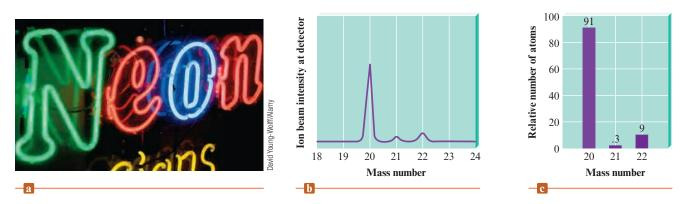
**Figure 3.2** (a) Neon gas glowing in a discharge tube. The relative intensities of the signals recorded when natural neon is injected into a mass spectrometer, represented in terms of (b) "peaks" and (c) a bar graph. The relative areas of the peaks are 0.9092 (<sup>20</sup>Ne), 0.00257 (<sup>21</sup>Ne), and 0.0882 (<sup>22</sup>Ne); natural neon is therefore 90.92% <sup>20</sup>Ne, 0.257% <sup>21</sup>Ne, and 8.82% <sup>22</sup>Ne.
