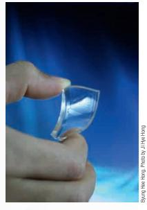
A flexible electrode made of graphene.
