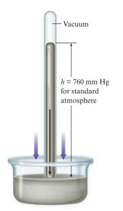
Figure 5.2 A torricellian barometer. The tube, completely filled with mercury, is inverted in a dish of mercury. Mercury flows out of the tube until the pressure of the column of mercury (shown by the black arrow) "standing on the surface" of the mercury in the dish is equal to the pressure of the air (shown by the purple arrows) on the rest of the surface of the mercury in the dish.
