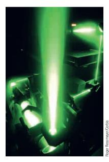
A Twyman–Green interferometer emits green argon laser light. Interferometers can measure extremely small distances, useful in configuring telescope mirrors.
