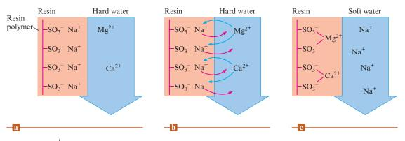
**Figure 20.6** (a) A schematic representation of a typical cation-exchange resin. (b) and (c) When hard water is passed over the cation-exchange resin, the  $Ca^{2+}$  and  $Mg^{2+}$  bind to the resin.
