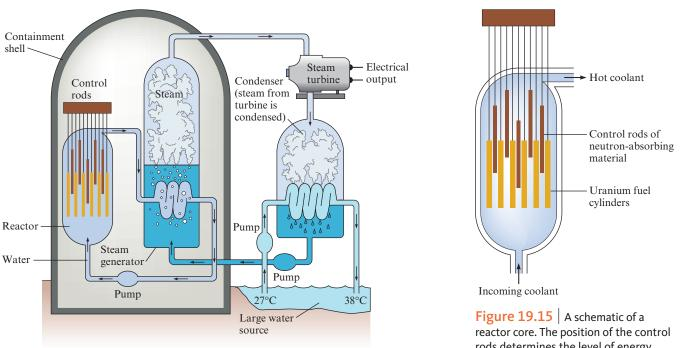
**Figure 19.14** A schematic diagram of a nuclear power plant.
