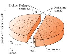
Figure 19.5 A schematic diagram of a cyclotron. The ion is introduced in the center and is pulled back and forth between the hollow D-shaped electrodes by constant reversals of the electric field. Magnets above and below these electrodes produce a spiral path that expands as the particle velocity increases. When the particle has sufficient speed, it exits the accelerator and is directed at the target nucleus.
