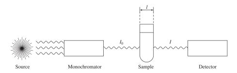
**Figure A.6** A schematic diagram of a simple spectrophotometer. The source emits all wavelengths of visible light, which are dispersed using a prism or grating and then focused, one wavelength at a time, onto the sample. The detector compares the intensity of the incident light ( $I_o$ ) to the intensity of the light after it has passed through the sample (I).
