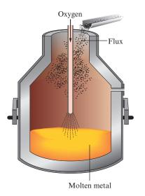
Figure 21.38 | The basic oxygen process for steelmaking.
