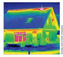
This infrared photo of a house shows where energy leaks occur. The more red the color, the more energy (heat) is leaving the house.
