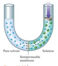
**Figure 11.20** Reverse osmosis. A pressure greater than the osmotic pressure of the solution is applied, which causes a net flow of solvent molecules (blue) from the solution to the pure solvent. The solute molecules (green) remain behind.
