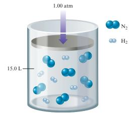
Assume this reaction mixture goes to completion. The piston apparatus allows the container volume to change in order to keep the pressure constant at 1.00 atm. Assume ideal behavior and constant temperature.
