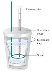
**Figure 6.5** A coffee-cup calorimeter made of two Styrofoam cups.
