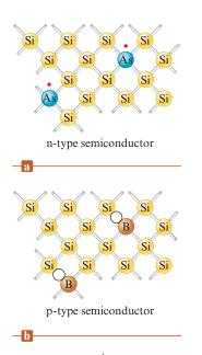
Figure 10.29 (a) A silicon crystal doped with arsenic, which has one more valence electron than silicon. (b) A silicon crystal doped with boron, which has one less electron than silicon.
