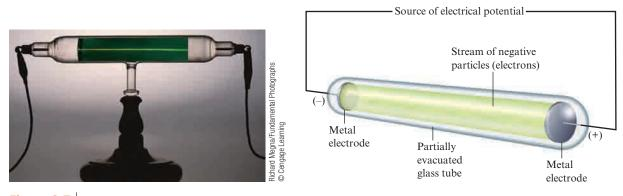
**Figure 2.7** A cathode-ray tube. The fast-moving electrons excite the gas in the tube, causing a glow between the electrodes. The green color in the photo is due to the response of the screen (coated with zinc sulfide) to the electron beam.
