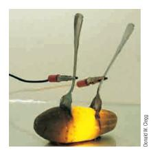
When alternating current at 110 volts is applied to a dill pickle, a glowing discharge occurs. The current flowing between the electrodes (forks), which is supported by the Na<sup>+</sup> and Cl<sup>-</sup> ions present, apparently causes some sodium atoms to form in an excited state. When these atoms relax to the ground state, they emit visible light at 589 nm, producing the yellow glow reminiscent of sodium vapor lamps.
