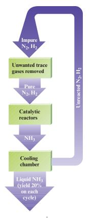
**Figure 20.12** A schematic diagram of the Haber process for the manufacture of ammonia.
