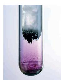
**Figure 10.41** | lodine being heated, causing it to sublime, forming crystals of  $I_2(s)$  on the bottom of a test tube cooled by ice.
