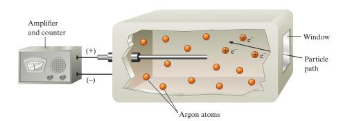
**Figure 19.7** A schematic representation of a Geiger–Müller counter. The high-energy radioactive particle enters the window and ionizes argon atoms along its path. The resulting ions and electrons produce a momentary current pulse, which is amplified and counted.
