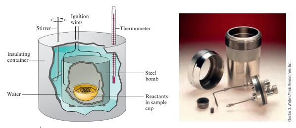
**Figure 6.6** A bomb calorimeter. The reaction is carried out inside a rigid steel "bomb" (photo of actual disassembled "bomb" shown on right), and the heat evolved is absorbed by the surrounding water and other calorimeter parts. The quantity of energy produced by the reaction can be calculated from the temperature increase.
