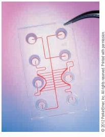
Plastic chips such as this one made by PerkinElmer, Inc. are being used to perform laboratory procedures traditionally done with test tubes.
