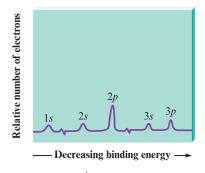
Figure 9.50 | The idealized PES spectrum of phosphorus.
