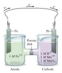
**Figure 18.7** The schematic of a galvanic cell based on the half-reactions:
