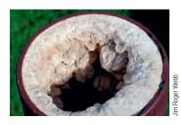
Figure 11.8 | A pipe with accumulated mineral deposits. The cross section clearly indicates the reduction in pipe capacity.
