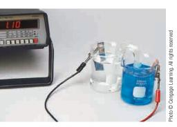
An electrochemical cell with a measured potential of 1.10 V.
