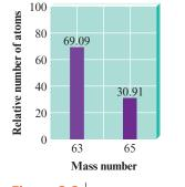
Figure 3.3 | Mass spectrum of natural copper.
