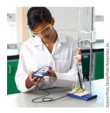
A setup used to conduct the pH titration of an acid or a base.
