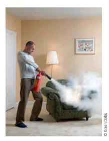
A carbon dioxide fire extinguisher being used to put out a fire.
