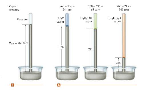
**Figure 10.38** (a) The vapor pressure of a liquid can be measured easily using a simple barometer of the type shown here. (b) The three liquids, water, ethanol ( $C_2H_5OH$ ), and diethyl ether [( $C_2H_5$ )<sub>2</sub>O], have quite different vapor pressures. Ether is by far the most volatile of the three. Note that in each case a little liquid remains (floating on the mercury).
