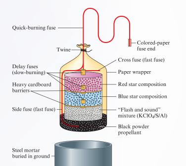
A typical aerial shell used in fireworks displays. Time-delayed fuses cause a shell to explode in stages. In this case a red starburst occurs first, followed by a blue starburst, and finally a flash and loud report. (Reprinted with permission from *Chemical & Engineering News*, June 29, 1981, p. 24. Copyright © 1981, American Chemical Society.)
