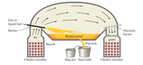
Figure 21.37 A schematic diagram of the open hearth process for steelmaking. The checker chambers contain bricks that absorb heat from gases passing over the molten charge. The flow of air and gases is reversed periodically.
