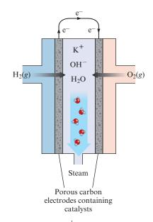
**Figure 18.16** | Schematic of the hydrogen-oxygen fuel cell.
