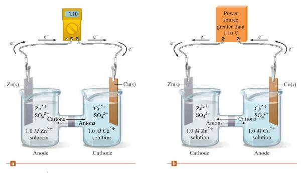
Figure 18.19 (a) A standard galvanic cell based on the spontaneous reaction  $Zn + Cu^{2+} \longrightarrow Zn^{2+} + Cu$
