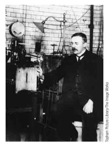
In 1909 Robert Millikan (1868–1953), working at the University of Chicago, performed very clever experiments involving charged oil drops. These experiments allowed him to determine the magnitude of the electron charge (Fig. 2.10). With this value and the charge-to-mass ratio determined by Thomson, Millikan was able to calculate the mass of the electron as  $9.11 \times 10^{-31}$  kg.
