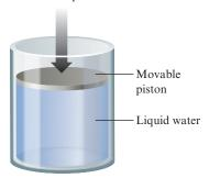
**Figure 10.45** Water in a closed system with a pressure of 1 atm exerted on the piston. No bubbles can form within the liquid as long as the vapor pressure is less than 1 atm.
