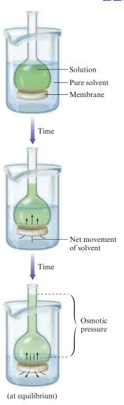
**Figure 11.16** A tube with a bulb on the end that is covered by a semipermeable membrane. The solution is inside the tube and is bathed in the pure solvent. There is a net transfer of solvent molecules into the solution until the hydrostatic pressure equalizes the solvent flow in both directions.
