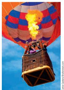
A propane burner is used to heat the air in a hot-air balloon.
