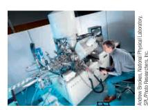
A researcher using a photoelectron spectrometer.
