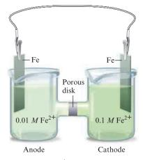
**Figure 18.10** A concentration cell containing iron electrodes and different concentrations of  $Fe^{2+}$  ion in the two compartments.
