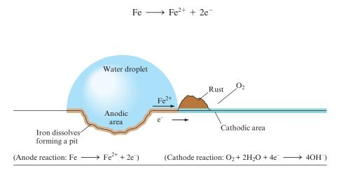
**Figure 18.17** | The electrochemical corrosion of iron.
