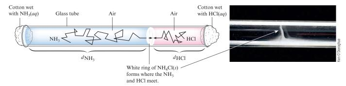
Figure 5.24 (above left) A demonstration of the relative diffusion rates of NH<sub>3</sub> and HCl molecules through air. Two cotton plugs, one dipped in HCl(aq) and one dipped in NH<sub>3</sub>(aq), are simultaneously inserted into the ends of the tube. Gaseous NH<sub>3</sub> and HCl vaporizing from the cotton plugs diffuse toward each other and, where they meet, react to form  $NH_4Cl(s)$ . (above right) When HCl(q) and  $NH_3(q)$ meet in the tube, a white ring of  $NH_4Cl(s)$  forms.
