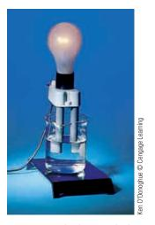
An acetic acid solution, which is a weak electrolyte, contains only a few ions and does not conduct as much current as a strong electrolyte. The bulb is only dimly lit.
