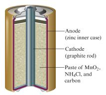
Figure 18.14 A common dry cell battery.
