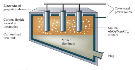
**Figure 18.22** A schematic diagram of an electrolytic cell for producing aluminum by the Hall–Heroult process. Because molten aluminum is more dense than the mixture of molten cryolite and alumina, it settles to the bottom of the cell and is drawn off periodically. The graphite electrodes are gradually eaten away and must be replaced from time to time. The cell operates at a current flow of up to 250,000 A.
