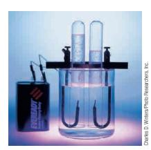
**Figure 18.20** | The electrolysis of water produces hydrogen gas at the cathode (on the right) and oxygen gas at the anode (on the left). Note that twice as much hydrogen is produced as oxygen.
