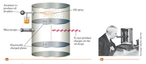
**Figure 2.10** (a) A schematic representation of the apparatus Millikan used to determine the charge on the electron. The fall of charged oil droplets due to gravity can be halted by adjusting the voltage across the two plates. This voltage and the mass of the oil drop can then be used to calculate the charge on the oil drop. Millikan's experiments showed that the charge on an oil drop is always a whole-number multiple of the electron charge. (b) Robert Millikan using his apparatus.
