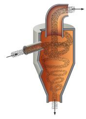
**Figure 21.34** A schematic diagram of a cyclone separator. The ore is pulverized and blown into the separator. The more dense mineral particles are thrown toward the walls by centrifugal force and fall down the funnel. The lighter particles (gangue) tend to stay closer to the center and are drawn out through the top by the stream of air.
