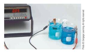
A concentration cell with 1.0 M  $Cu^{2+}$  on the right and 0.010 M  $Cu^{2+}$  on the left.
