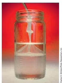
Figure 22.16 The reaction to form nylon can be carried out at the interface of two immiscible liquid layers in a beaker. The bottom layer contains adipoyl chloride,
